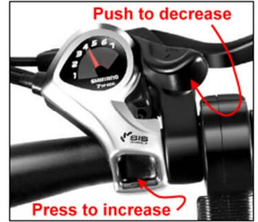
**NEVER SHIFT** unless you are pedaling. Do not shift while sitting, coasting, or throttle-only. You must be pedaling. We recommend 3<sup>rd</sup> or 4<sup>th</sup> gear most of the time.
